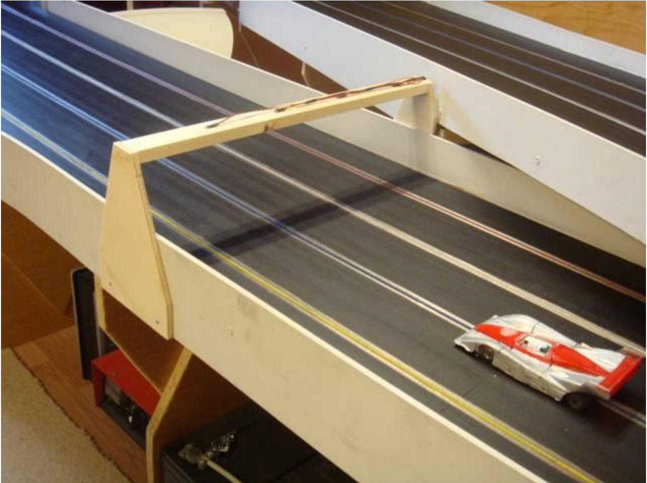
IR-Sensor Bridge installed at the LapMaster test track.
